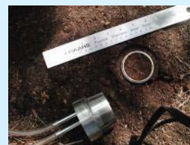
II. A 2 1/4" Soil Core in Soil & PMAP Air-Space Cap
