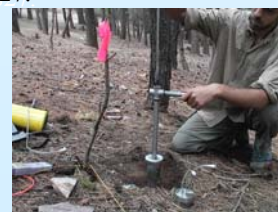
I. Soil Core Sampler Pounded to a depth of 4"
